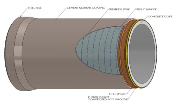
PRESTRESSED CONCRETE LINED CYLINDER PIPE for sizes below 1400 mm
