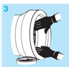
Lubricate bell jointing surface liberally. Use a brush, cloth, sponge or gloves to cover entire surface. Only approved lubricant should be used.
