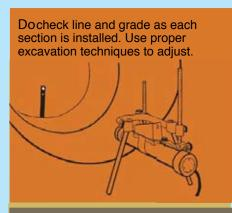
Don't push, pound or rock installed pipe with excavator bucket to establish grade.
