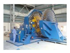
MBK Cage Welding Machine can make cages in diameters ranging from 300 millimeters to 3600 millimeters.
