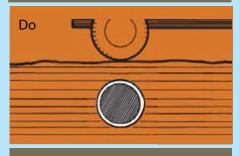
Don't operate heavy construction equipment over the pipe until adequate cover is in place.
