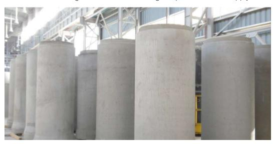
Lining of concrete pipes with various materials available in market today via., HDPE, PVC or GRP make these the most suited pipes to withstand many kinds of aggressive fluid flows which even steel pipes may fail to offer in the longer run.
