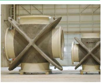
The pipes are used generally for pressure flow applications, a large variant of pressure ratings are offered. Standard pipes can be offered up to 25 Bar pressure and above that project specific details are provided on request.
