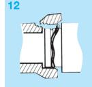
Unequal stretch could cause bunching of gasket and may cause leaks in the joint or crack the bell.
